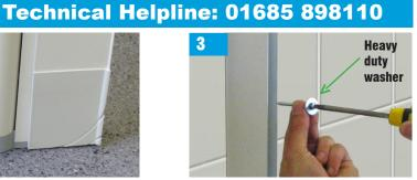
Drill holes in the wall with a No10 masonry drill bit, insert wall plugs, and fix with the No8 x 50mm pan head wood screws and heavy duty washers provided.
