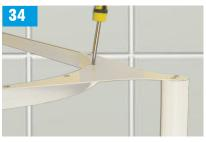
Screw the boomerang bracket to the curtain rail using the No6 x  $\frac{3}{4}$ " countersunk screws. **USE THE SCREWS PROVIDED.**
