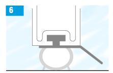
Ensure that the rubber seal on the bottom of the door(s) is slightly compressed against the tray surface or floor.
